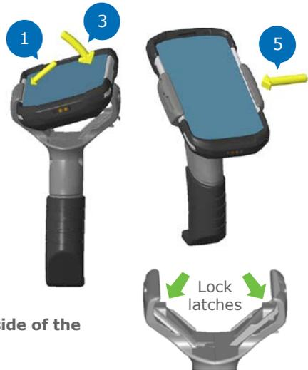
Now press down the left and right hand side of the retaining clip until it snaps.
