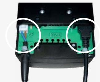
Protected plugs and simple cable protection (example: supply and USB cables)
