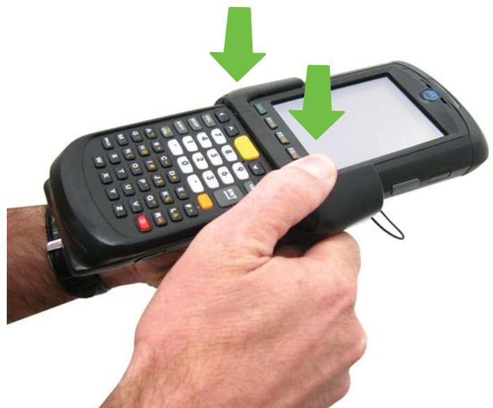
Now press down the left and right hand side of the retaining clip until it snaps.
