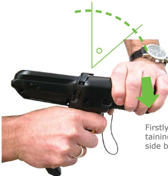
Firstly release the brackets of the retaining clip on the left and right hand side by pushing them firmly.
