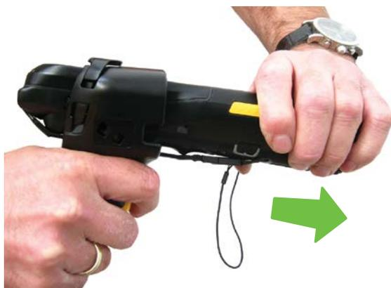
Now pull the device forwards and remove it from the TISPLUS Scan Handle.
