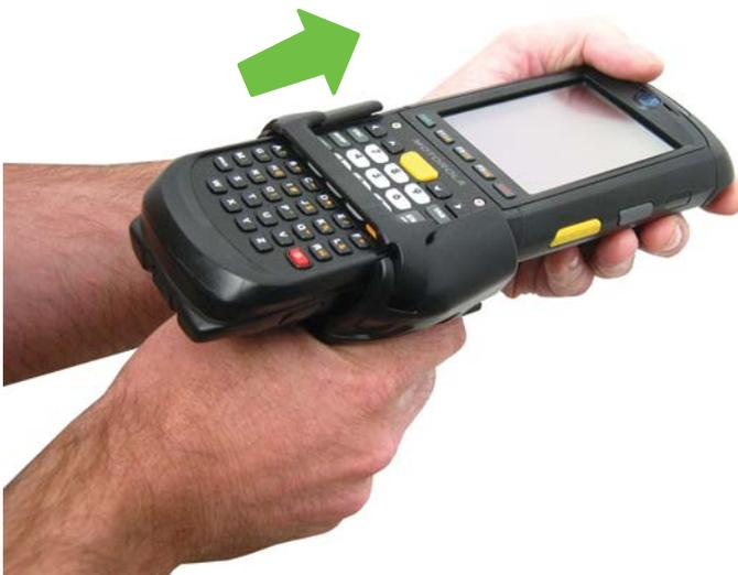
Push the TISPLUS Scan Handle onto the device until you hear a snapping sound.
