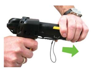
Now pull the device forwards and remove it from the TISPLUS Scan Handle.
