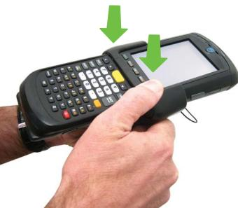
Now press down the left and right hand side of the retaining clip until it snaps.
