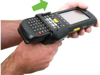
Push the TISPLUS Scan Handle onto the device until you hear a snapping sound.
