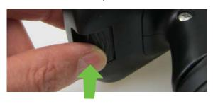
Now pull the device forward and remove it from the TISPLUS Scan Handle.
