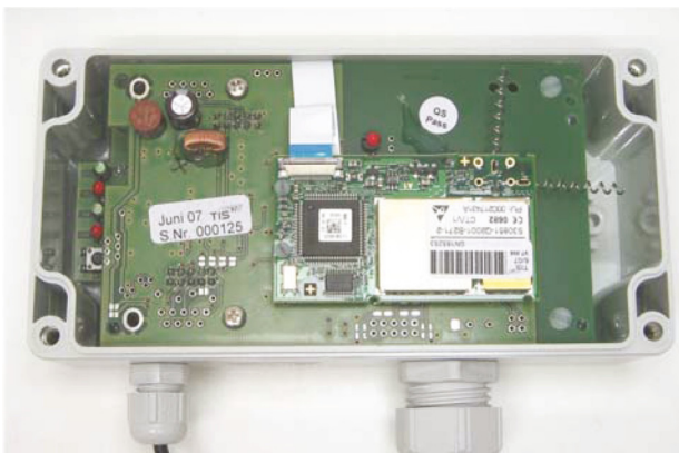
Fig. 1: DECT module with internal antenna
